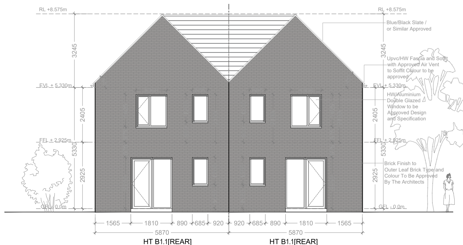
07 102 REAR ELEVATION 1:100 BLOCKS 6&9
